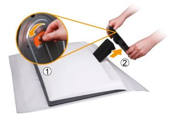
After placing the monitor panel on a soft cloth or cushion, complete the following steps to remove the base.
